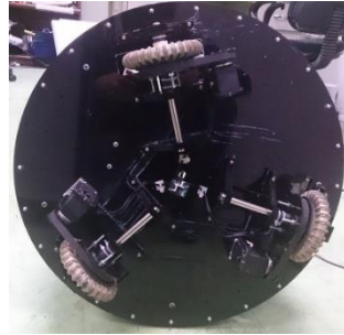
Fig. 1. This figure shows Sepanta's motion mechanism which contains three omni-directional wheels.
